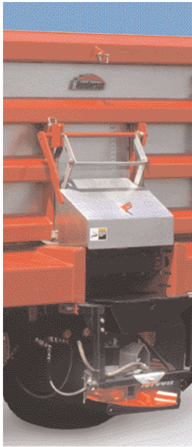
REAR CENTER Distribution is from the rear center of the body. Material is fed by a conveyor and is spread behind the truck.
