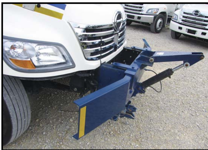
Straight-through (not bolted-on) frame rails extend 23 inches forward of the nose to accommodate the plow mount. Heavy steel plow adds to the weight on the front end, so the Meritor steer axle's capacity is 14,000 pounds.
