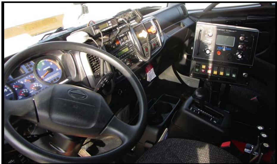
Interior is a pleasant but busy place, with radios on the dash and controls for the box, sander and plow taking space to the driver's right. Allison lever-type selector reads R-N-D-5-4-3-2-1, so driver can catch just the gear he needs during plowing and other work.
