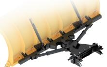
**Outboard Cylinders Push Frame** STANDARD OR FULL-WIDTH
